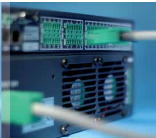
“Plug and play” installation: VA/PA systems from ESSER can be easily connected by plugs; no extensive cabling is necessary.
